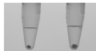
Fig. 1: recommended pellet sizes Left: maximum pellet size for turbidity from bacteria Right: maximum pellet size for yeast turbid samples
