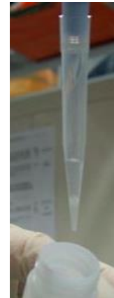
Fig. 2: recommended volume of beads per Lysis buffer in the pipette tip
