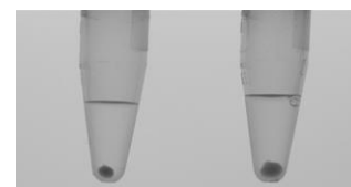
Fig. 1: recommended pellet sizes Left: maximum pellet size for mold Right: pellet size too large
