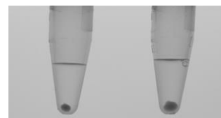
Fig. 1: recommended pellet sizes Left: maximum pellet size for turbidity from bacteria Right: maximum pellet size for yeast containing samples
