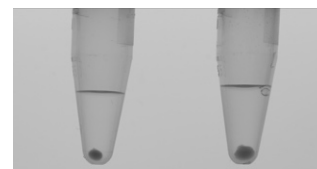
Fig. 1: recommended pellet sizes Left: maximum pellet size for turbidity from bacteria Right: maximum pellet size for yeast containing samples
